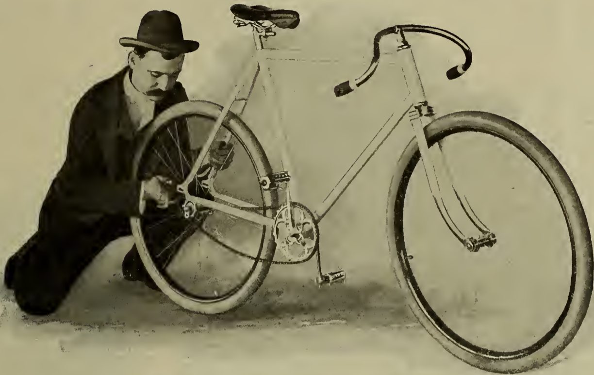
Removing Rear Wheel from Frame Without Disturbing Adjustments or Detaching Chain.
